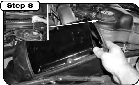
Step 8 Remove two screws holding the radiator overflow reservoir. Install aFe filter box, radiator overflow reservoir will need to be slightly shifted to the side to allow enough room for filter box to drop into place.
