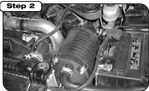
Step 2 Complete stock intake. Disconnect battery terminals to reset computer.
