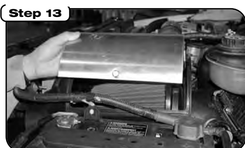
Step 13 Install filter into housing and tighten clamp. Install aluminum housing lid with the aFe logo facing towards the front of the vehicle. Tighten captive screws with a snug fit.
