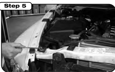
Step 5 Using 10 mm wrench, remove the bolt that secures the factory airbox to the radiator bulkhead.
