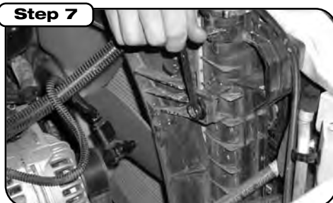
Step 7 Using a 13mm wrench, loosen and remove the upper passenger-side bolt on the radiator shroud and set aside for installation of heat shield. Verify that the engine is cool, then temporarily remove the overflow hose from the radiator filler neck for clearance.
