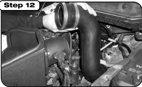
Step 12 With clamps and couplers provided install high temp coupler at turbo side and 4"x3" urethane coupler at filter side, tighten using 5/16" nut driver. Install pre-oiled filter onto intake tube and tighten. Do not use any oil or grease when attaching filter. Reattach radiator overflow hose that was removed in Step 7.
