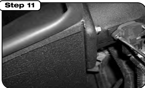
Step 11 Install intake temperature sensor that was removed from the airbox onto the aFe intake tube using provided hardware and gasket, then tighten. Orientation does not matter on the temperature sensor. Re-connect factory harness to the temperature sensor.
