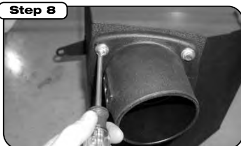
Step 8 Install aFe intake tube and trim seal on the heat shield, be sure to install in the orientation shown. Install heat shield into engine compartment but do not attach any bolts. The bottom louvered panel must be positioned above the aluminum A/C line.
