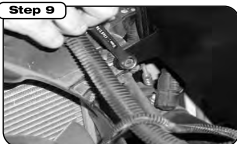
Step 9 Using the bolt removed from the fan shroud earlier, secure the heat shield to the shroud using the tab extending from the heat shield, do not fully tighten.
