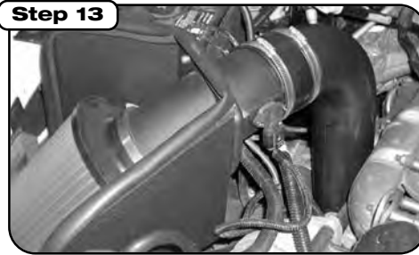
Step 13 Complete intake kit installed. Be sure to re-check connections and re-tighten after a few hours of operation. Thank you for choosing aFe!
