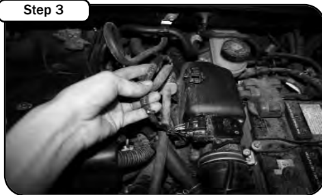
Disconnect MAF sensor. Remove vacuum lines away from upper half of air box. Disconnect the factory clips holding the air box in place.
