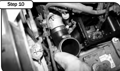
Install 2-1/2" elbow coupler onto throttle body with #040 clamps provided.
