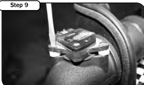
Insert MAF sensor with gasket, 1/4" nylon spacer and M4 screws provided between sensor and tube. Tighten using flathead screwdriver.
