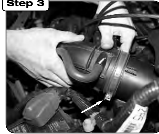
With phillips screwdriver, loosen OE intake tube clamp @ airbox and pull away.
