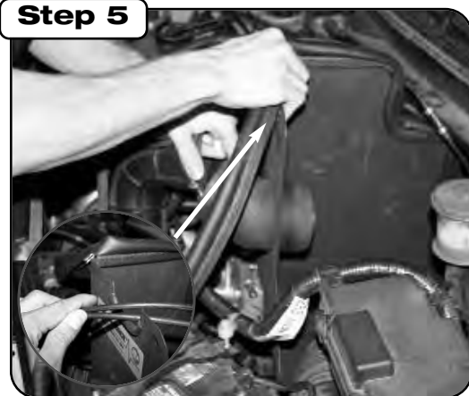
Install new housing into vehicle. Place 3-1/2L" rubber edge trim in groove above Magnum Force decal. Have both cable lines between groove in housing. Now install 3/4" trim seal to housing.
