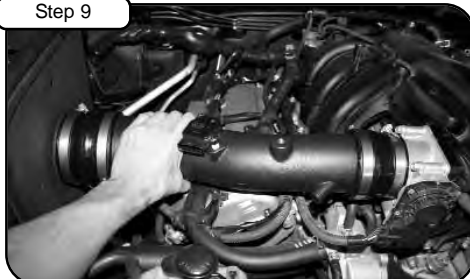
Place couplers on to tube with clamps provided, and install loose to allow repositioning. DO NOT TIGHTEN CLAMPS!
