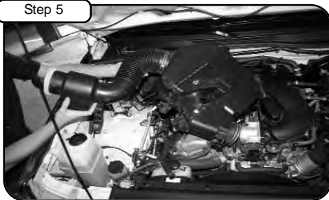
Disconnect fuel regulator line and valve cover vent line. Remove OE intake out of vehicle.
