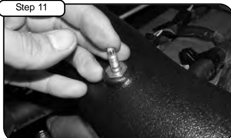
Remove M6 insert from OE airbox, loosen using adjustable wrench. Re-install onto new tube and tighten.
