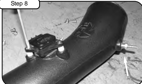
Remove MAF sensor from OE airbox using philips screwdriver. Re-install to new aFe tube with hardware provided ( make sure gasket and nylon spacers are between tube and sensor ) using flat head screwdriver. Install brass hose fitting.
