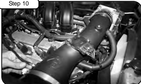
Re-connect MAF sensor harness, valve cover vent line, and fuel regulator with 5/32" hose provided.
