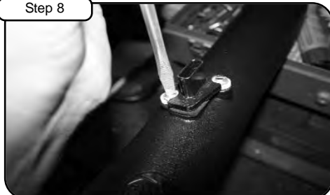
Remove MAF sensor from OE airbox using phillips screwdriver. Re-install to new aFe tube with hardware provided (make sure gasket and nylon spacers are between tube and sensor) using flat head screwdriver.
