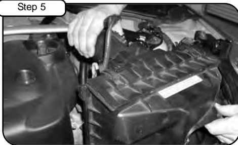
Carefully lift, and remove OE airbox out of vehicle.
