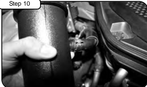
Re-install crank case breather to new tube.
