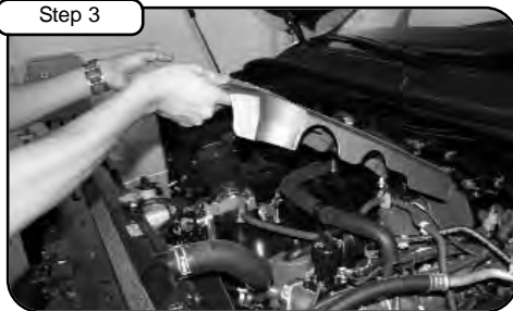
Lift up and remove engine cover.
