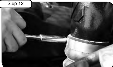
Step 12 Tighten coupler hose clamp with 11mm socket (See notes 2 & 4). Tighten the four mounting bolts from Step 11 (See notes 2 & 5).
