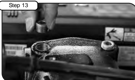
Step 13 Install the two 3/8" NPT plugs to top of aFe manifold. Tighten using 8mm allen key (See notes 1, 2 & 5).
