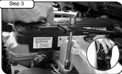
Step 3 With 10mm socket and extension, remove the 4 bolts holding the stock manifold. Remove the engine wiring harness connections in back of stock manifold. Pull harness bracket off mounting stud.
