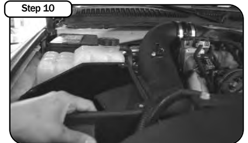
Place hump coupler at end of tube with clamps provided. Install into vehicle. Position tube and housing to factory position. Do not tighten clamps!
