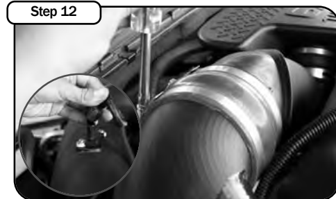
Tighten clamps @ turbo end with 5/16" nut driver. Re-connect MAF sensor harness.
