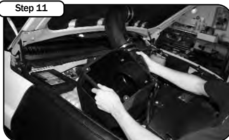
Install into vehicle. Position tube and housing to factory position. Do not tighten clamps!
