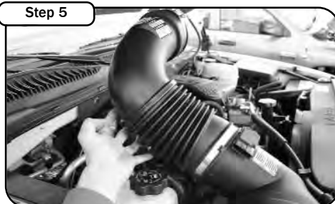
Carefully grab and pull out OE intake system. Remove out of vehicle.
