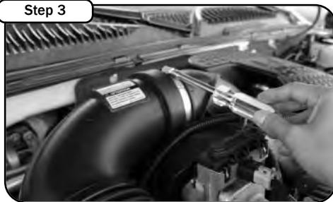
With 5/16" nut driver, loosen the clamp @ turbo end.
