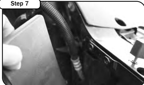
Remove plastic cover behind passenger head light.
