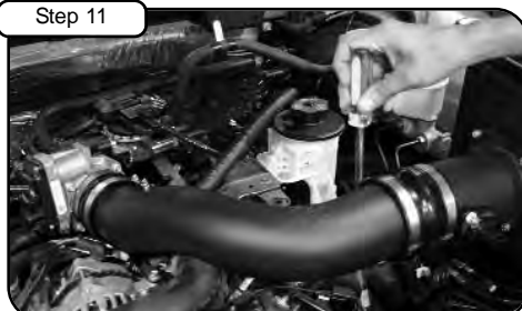
Step 11 Install new tube to throttle body and intake housing. Tighten clamps with 5/16" nut driver. Finish install on crank case line with mini clamp and tighten.
