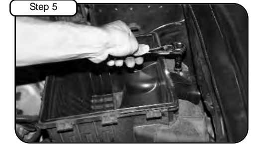
With 10mm socket or wrench loosen the 2 screws holding in OE air box. Lift up and remove OE air box out of vehicle.
