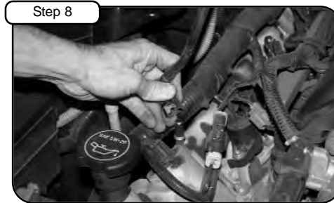
Remove factory crank case line from engine.
