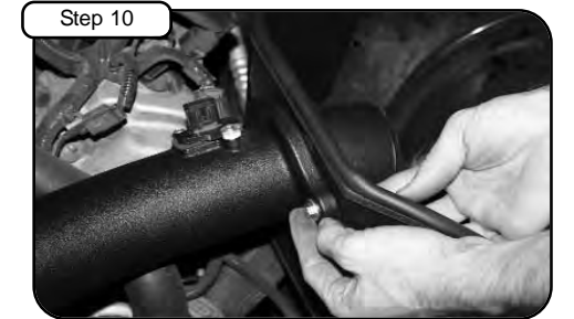
Install screws/nuts and washer provided to mount tube to housing. Tighten using 10mm socket or wrench.
