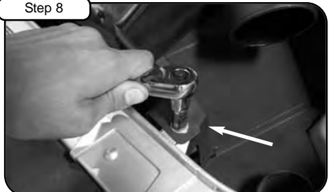
Tighten down housing using OE bolt. Use 10mm socket or wrench.
