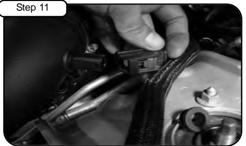
Re-connect air temp sensor harness.
