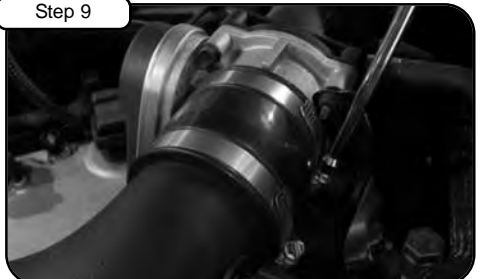
Tighten clamps using 5/16" nut driver.
