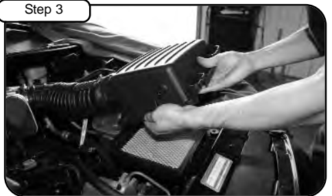
Disconnect air temp sensor and crank case line. Lift up and pull OE air box out of vehicle.
