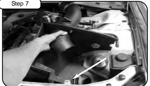
Install intake into vehicle. Position housing to tab.
