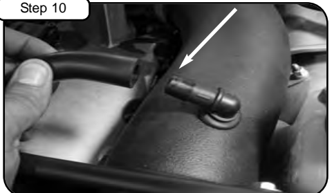
Re-connect crank case line to fitting on tube.
