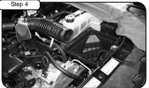
Loosen and remove OE intake tube with 5/16" nut driver. Remove bottom air box out of vehicle. Remove air temp sensor.
