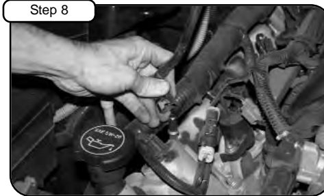
Remove factory crank case line from engine.
