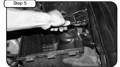
With 10mm socket or wrench loosen the 2 screws holding in OE air box. Lift up and remove OE air box out of vehicle.
