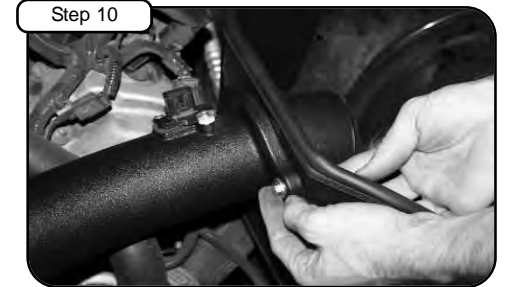
Install screws/nuts and washer provided to mount tube to housing. Tighten using 10mm socket or wrench.
