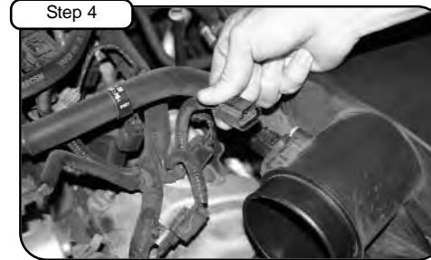
Disconnect MAF sensor harness.
