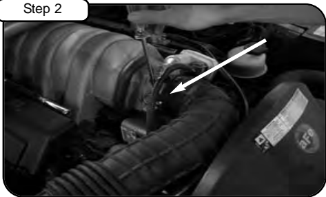
With 5/16" nut driver loosen the clamp on throttle body side.
