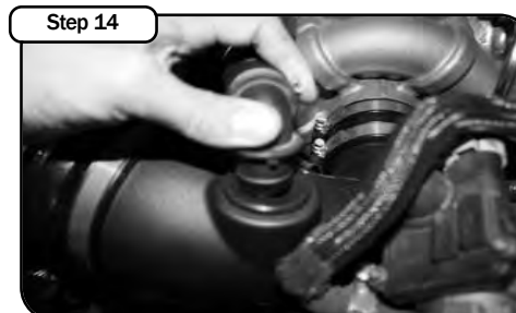
Re-install crank case line into new tube. Push down completely. Re-connect MAF sensor and filter minder.
