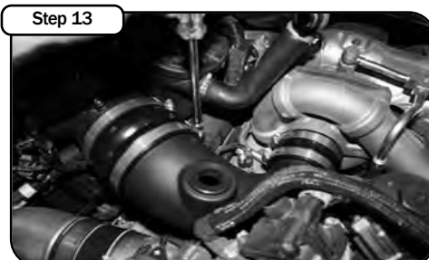
Install new tube with couplers and clamps provided. Tighten using 5/16" nut driver. Install grommet into tube.
