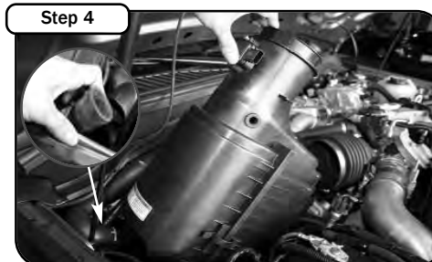
Take auxillary air line out of air box. Lift and pull firmly then remove OE air box out of vehicle.
