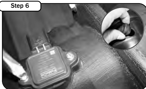
With T-20 torx bit provided loosen the two bolts holding in MAF sensor and remove. Remove grommet for filter minder. With screws and gasket provided, install MAF sensor into new intake tube. (make sure gasket is between sensor and tube) Re-install filter minder grommet into intake tube.
