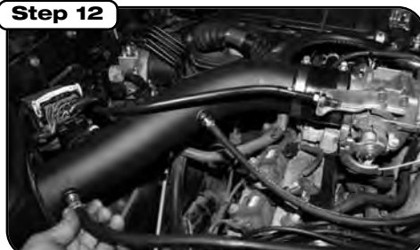
Step 12 Remove large diameter vent hose still connected to the throttle body and small diameter vacuum hose, retain factory evap hose (closest to heat shield.) Replace removed hoses with hoses in kit and connect all hoses to intake tube; clamps are not necessary.
