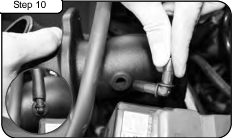
Install tube into housing and place 3/8" fitting into tube. Now install 3/8" hose to fitting.
