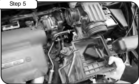
Remove complete air box out of vehicle.
