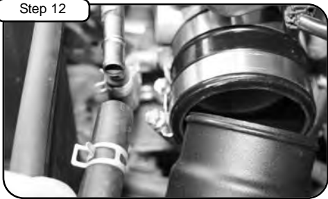
Install coupler with clamps to throttle body. Place 3/8" hose to metal vacuum line with OE clamp. Position tube to coupler and holes on housing. Do not tighten clamps.
