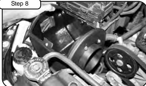
Install housing into vehicle. Use factory screw from step 5 to mount tab on new housing.
