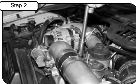
Step 2 With a 7/16" socket with ratchet, loosen the intercooler coupler hose clamp. See note 6.
