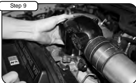
Step 9 Carefully guide manifold into coupler hose.
