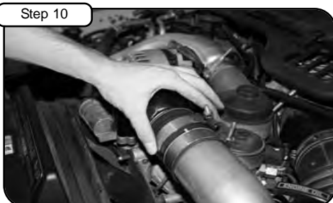
Step 10 Slide back clamp. Do not tighten.
