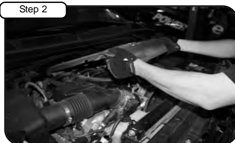
Remove engine cover by grasping as shown and carefully lifting up.
