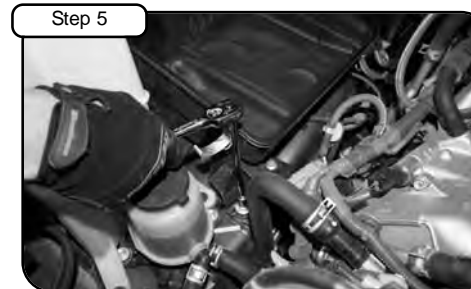
With 12mm socket or wrench loosen the 3 bolts holding in air box. Remove complete air box out of vehicle.
