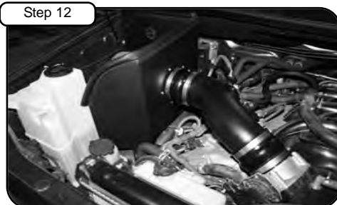
Tighten all clamps with 5/16" nut driver. Re-connect MAF sensor harness. Re-install engine cover.
