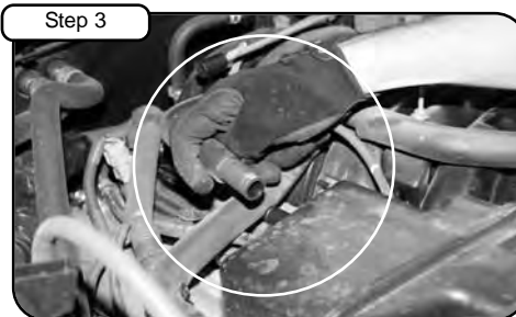
Disconnect vacuum line. Remove crankcase line out of vehicle. Disconnect MAF sensor harness.
