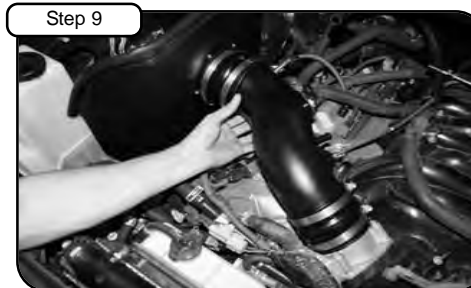
With couplers and clamps provided install new tube into vehicle. Position tube to throttle body and housing.
