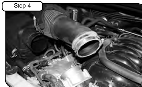
Remove OE intake tube. Un-clip upper half of air box and remove air filter.
