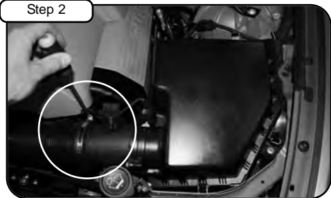
Disconnect MAF sensor harness. Loosen clamps with 1/4" nut driver.
