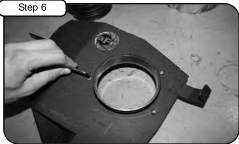
Install filter adaptor using 3 button head screws & wavy washers. Tighten using 5mm allen key.
