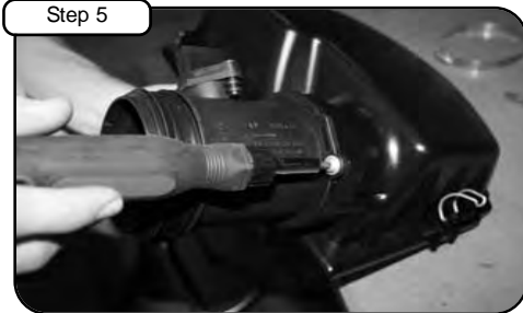
Remove MAF sensor using T30 torx bit.
