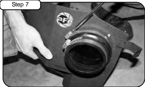
Install coupler reducer to filter adapter with clamps provided.
