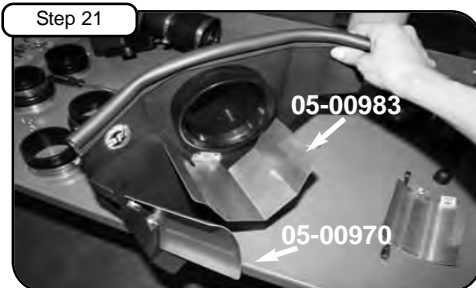
Attach air diverters to housing using button head and wavy washers. Tighten using 5mm allen key. Install 3/4" trim seal on housing. Install small 7/16" trim seal to corner of housing. Note: Failure to install air diverters may result in CEL (Check Engine Light).
