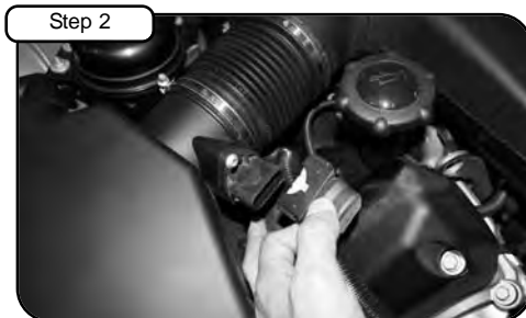
Step 2 Disconnect MAF sensor harness. Loosen clamps with 1/4" nut driver.
