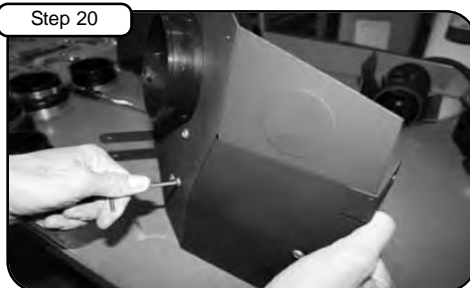
Attach filter adaptor to housing using 3 button head screws & wavy washers. Tighten using 5mm allen key.
