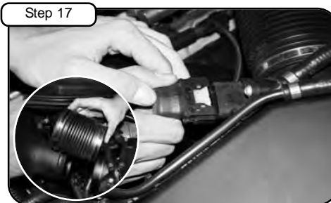
Disconnect MAF sensor harness. Loosen clamps with 1/4" nut driver. Take out plastic intake tube.
