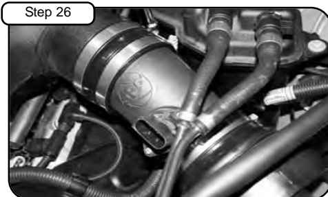
Position tube and tighten all clamps using 5/16" nut driver.
