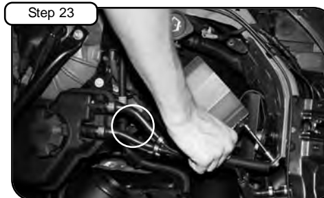
Re-install nut from step 4 and tighten using 10mm socket or wrench.
