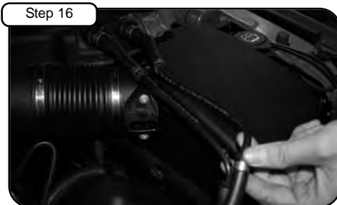
Pull out lines on top of air box.
