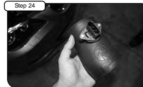
Remove MAF sensor from airbox and install in new tube (05-00969) with screws and gasket provided. Tighten using flathead screwdriver.
