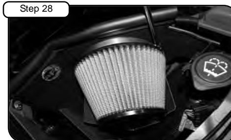
Install air filter and tighten using 5/16" nut driver. Install pre filter. Make sure cap is installed in filter top. Re-connect MAF sensor harness.
