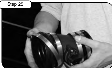
With couplers and clamps provided, install tube into vehicle.
