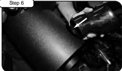
Step 6 Place coupler into housing using guides to seat in hole.
