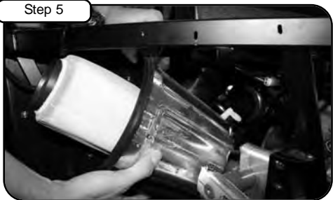
Step 5 Remove air box from intake tube.
