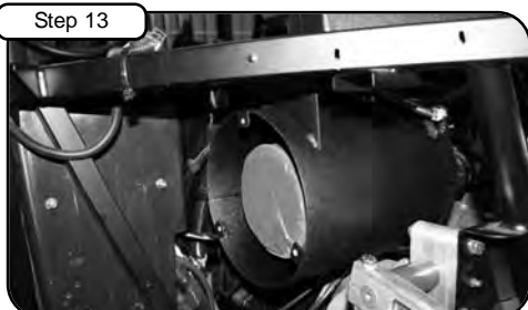
Step 13 Tighten clamp through slot on side of housing using 5/16" nut driver.
