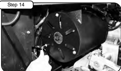
Step 14 Attach cover to housing, using button head screws and wavy washers provided and tighten using 5/32" allen key.
