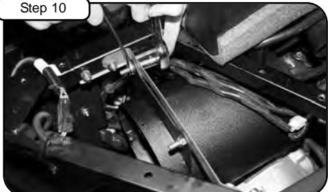
Step 10 Tighten all screws with 7/16" socket and wrench.
