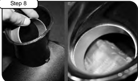
Step 8 Install aluminum ring inside coupler. Place ring inside of coupler from top, push and set between coupler and housing.
