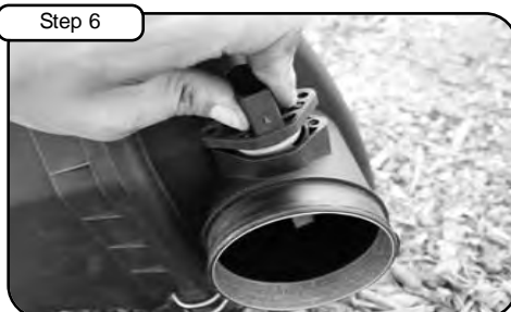
Remove MAF sensor from stock air box using T20 torx bit.
