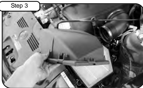
Unclip upper half of air box and lift carefully.
