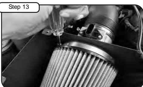
Install air filter and tighten using 5/16" nut driver. Tighten clamps on intake tube using 1/4" nut driver.
