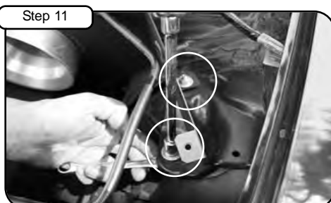
With screws, washers and nuts provided, place through holes from step 5. Tighten using 10mm socket or wrench.
