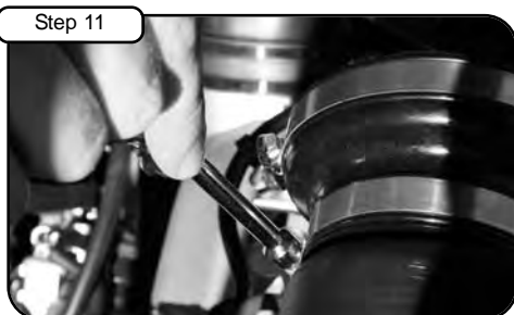
Tighten clamps on coupler using 5/16" nut driver.
