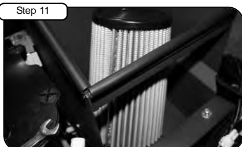
Install air filter onto housing. Do not tighten. This prevents anything from falling into intake tract.
