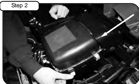
Un-clip upper half of air box with OE air filter and remove.
