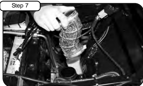
Remove OE intake tube out of Rhino.
