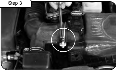
Loosen clamp on air box with 10mm socket or wrench.
