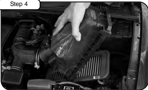
Unclip the side of air box. Remove upper half of air box. Remove air filter.
