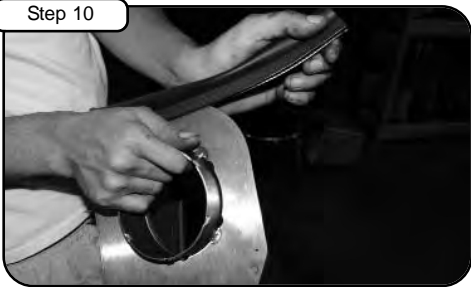
Attach trim seal to housing.
