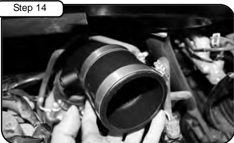
Install Throttle Body Tube (05-00808) tube along with coupler (05-00418) and clamps. Do not tighten.
