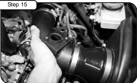
Install MAF tube (05-00997) with coupler (05-00649) and clamps on housing side. Position all tubes and tighten clamps using 5/16" nut driver.
