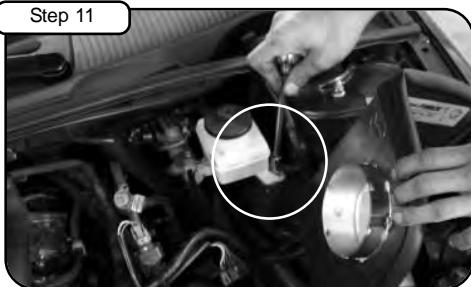
Loosen bolt holding in brake fluid reservoir. Install housing and position (see step 12).
