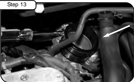
Install coupler (05-00417) to Throttle Body with clamps provided. Tighten clamp on Throttle Body only.
