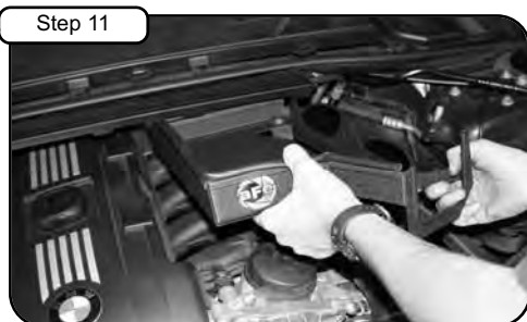
Install housing into factory position.
