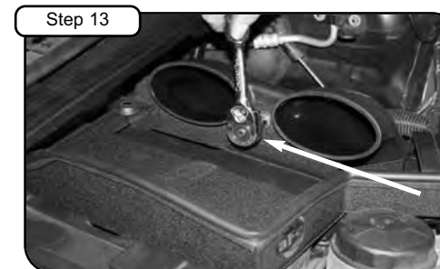
Install screw, washer and wavy washer provided, and tighten with 10mm socket or wrench. Tighten clamps to tube with 1/4" nut driver.
