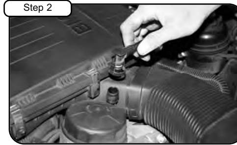
Disconnect vacuum line and pull back.
