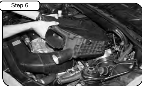
Remove complete air box from vehicle.
