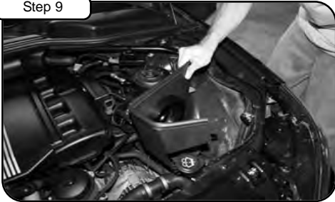
Attach trim seal to housing. Install housing into vehicle and position.
