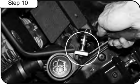
Secure housing using bolt from step 8 and tighten using 10mm socket or wrench.
