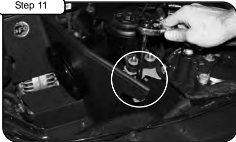
With bolt from step 4A, tighten down housing using 10mm socket or wrench.
