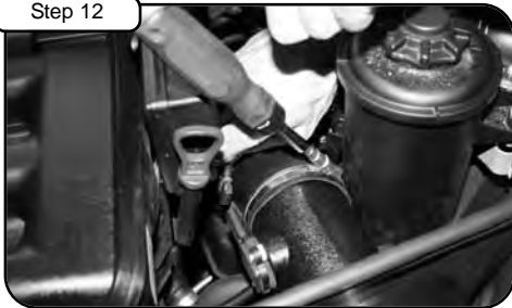
Attach stock tube to intake. Pull stock tube, hold, and tighten clamp using 1/4" nut driver. Connect MAF sensor harness.
