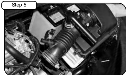
Step 5 Un-clip upper half of air box and remove with intake tube. Remove air filter.
