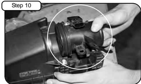
Step 10 Gently pull out MAF sensor from air box.
