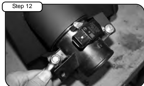
Step 12 With M6 screws, washers, lock washers, and nuts provided, tighten down MAF sensor to brackets on housing using 10mm socket or wrench.
