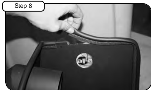
Step 8 Install 7/16 trim seal on housing.
