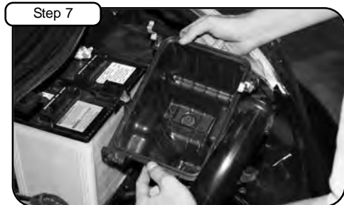
Step 7 Remove bottom half of air box.
