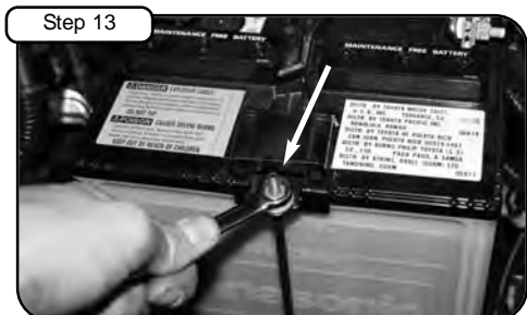
Step 13 Loosen nut holding in battery bracket and set aside for later install of housing (see step 20).
