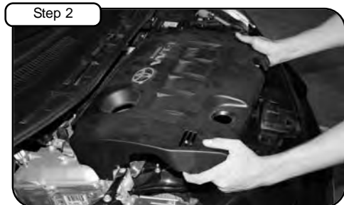
Step 2 Remove engine cover by lifting up front of cover and pulling up.
