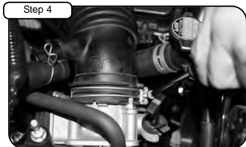
Step 4 Loosen clamp on Throttle Body with phillips screwdriver or 10mm socket or wrench.
