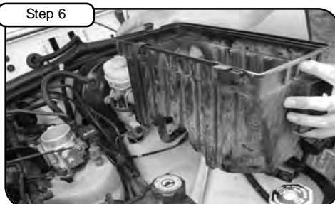
Step 6 Remove air box from vehicle.
