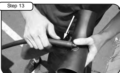
Step 13 Install 1/2" hose on fitting.
