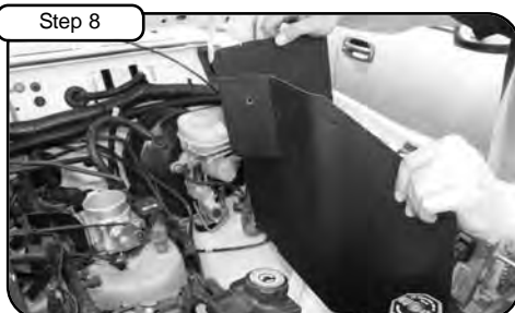
Step 8 Place housing in vehicle and position holes of housing in factory positions.
