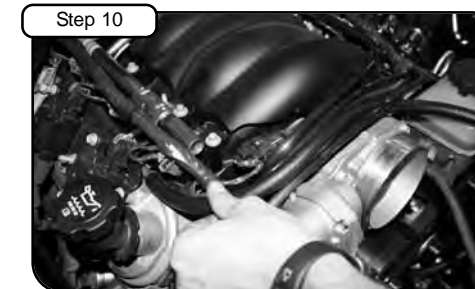
Step 10 Replace crankcase line with new 3/8" hose provided to engine and position like factory hose from step 9.
