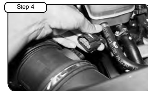
Step 4 Disconnect MAF sensor harness.
