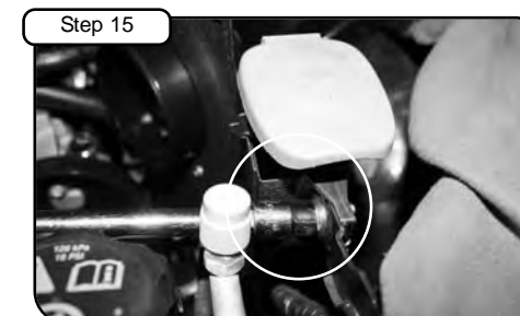
Step 15 With new screw, wavy & flat washers provided, tighten down housing tab to washer reservoir.
