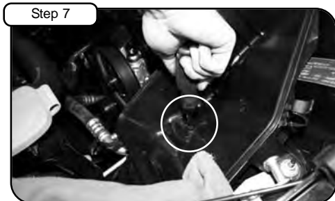
Step 7 Loosen bolt on bottom of air box with T27 torx bit and remove.
