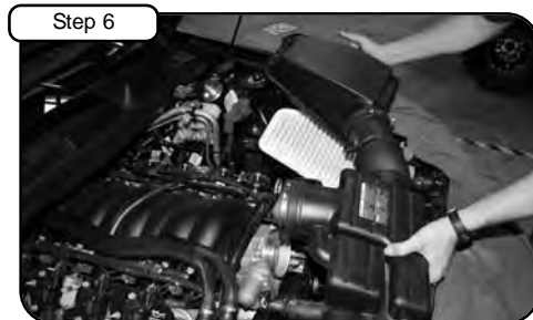
Step 6 Remove tube/sensor/upper air box in one piece. Remove stock air filter.
