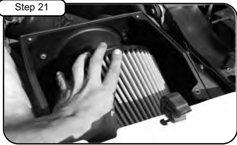
Step 21 Install air filter to tube. Make sure filter seats on tube bead.
