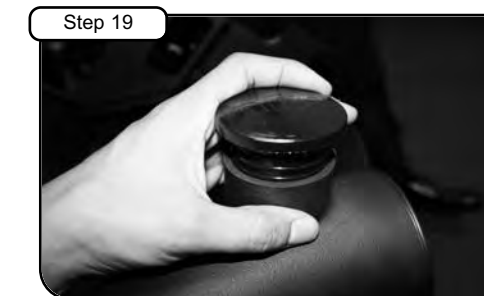
Step 19 If vehicle does not come equipped with resonator box, use aFe urethane plug on tube.
