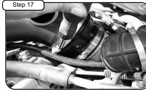
Step 17 Tighten reducer coupler clamps with 5/16" nut driver.
