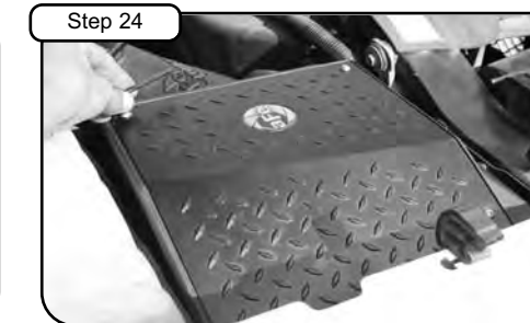
Step 24 Tighten cover using button head screws provided using 5/32" allen key.
