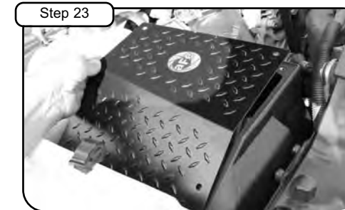
Step 23 Attach cover to housing.
