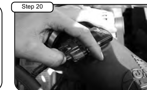
Step 20 Re-connect MAF sensor harness.
