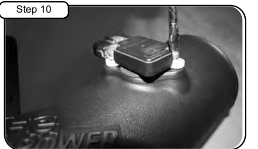
Install MAF sensor into new tube. Use provided screws, nylon spacers and gasket and tighten using flat head screwdriver.
