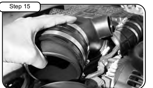
Install tube to turbo inlet flange and position. Make sure reducer coupler is on turbo flange. Do not tighten.
