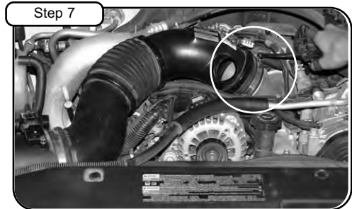
Loosen clamp on turbo with 5/16" nut driver.
