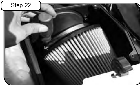
Step 22 Tighten air filter using 5/16" nut driver.
