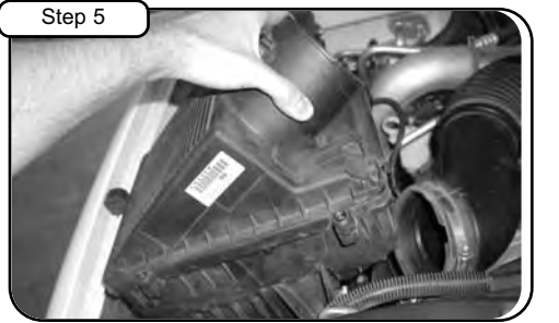
Lift and pull air box out of vehicle.
