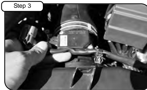
Step 3 Disconnect MAF sensor harness and pull clips away from air box.
