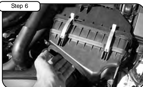
Step 6 Carefully grab front of air box from ram air unit and lift.
