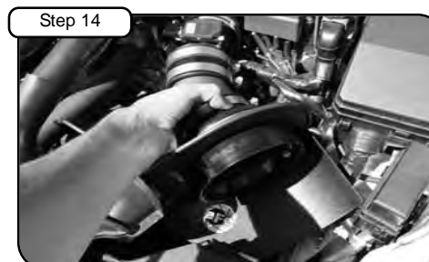
Step 14 Install intake assembly shown in step 13 into vehicle and position.
