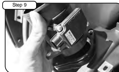
Step 9 Remove MAF sensor tube assembly from air box.
