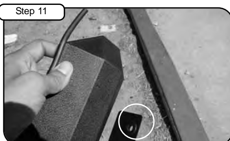
Step 11 Install rubber edge trim seal to top of housing. Install grommet to hole on housing..
