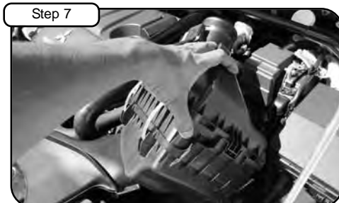
Step 7 Lift and pull out complete air box.
