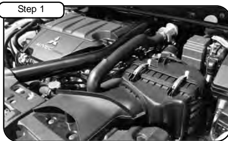
Step 1 Complete Stock Intake. Disconnect battery before install.
