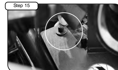
Step 15 Push down housing for rubber grommet to sit on factory tab.
