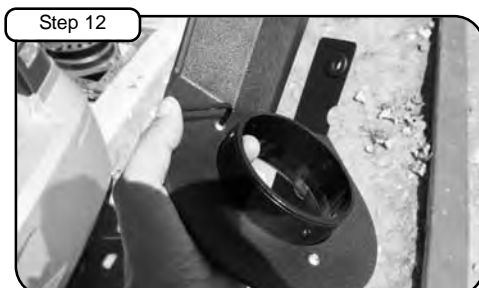
Step 12 Install filter adaptor to inside of housing. Attach to housing using the 3 button head screws provided and tighten using 6mm allen key.
