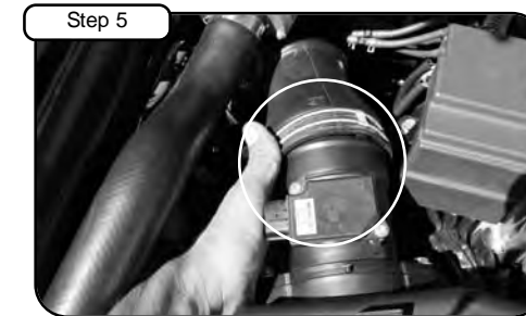
Step 5 Pull stock tube away from MAF sensor.
