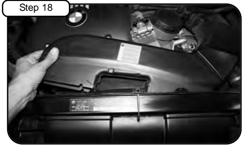
Pull back ram air duct and remove.
