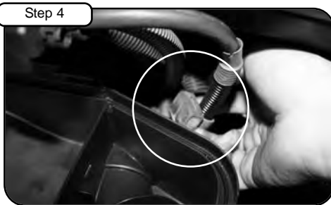
Pull back rubber mount attached to battery cable. Use pliers if necessary. This will allow stock clamp to be loosened. (To be done in step 5B.)
