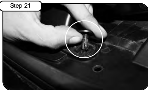
Remove plastic clip. Repeat steps 19-21 for remaining clip. (Save for later installation)
