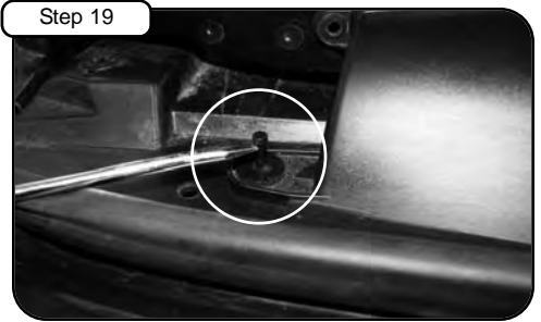
With flat head screwdriver, carefully pry and push up plastic pin.
