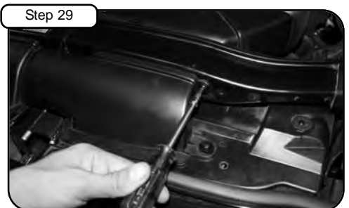
Re-position ram air duct from step 3. Secure using the 2 screws from step 17 and tighten using T25 torx bit.
