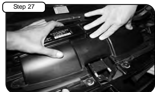
Have person B re-install the cover and secure with plastic pin clips that were removed earlier. (See steps 19-21)
