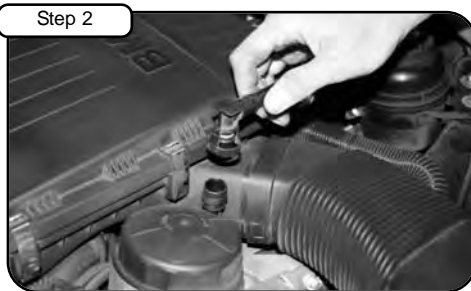
Disconnect vacuum line and pull back.
