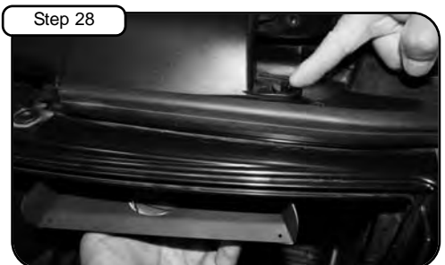
Detail of properly installed plastic pin clips. Make sure pin clips are through hole on scoops allowing to secure and hold in place!
