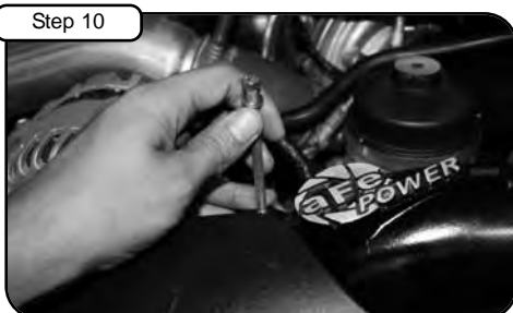
Install and secure manifold using 2 M6 x 1.00 x 100 screws and washers provided and tighten loosely.
