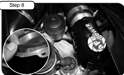
Install 1/8" NPT plugs to back of manifold. Tighten using 3/16" allen key. Attach new seal ring to bottom of manifold. Install new aFe BladeRunner manifold to vehicle. See Notes 2 & 3.
