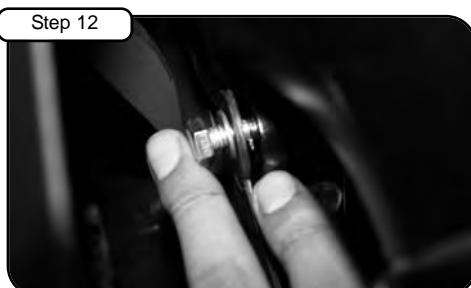
Attach screw through fan shroud hole and tighten to manifold. See Notes 2 & 5
