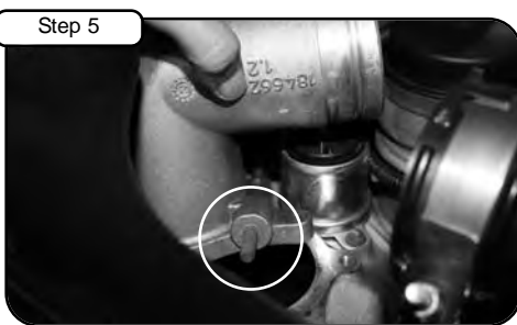
Pull back manifold screw away from fan shroud and remove manifold.
