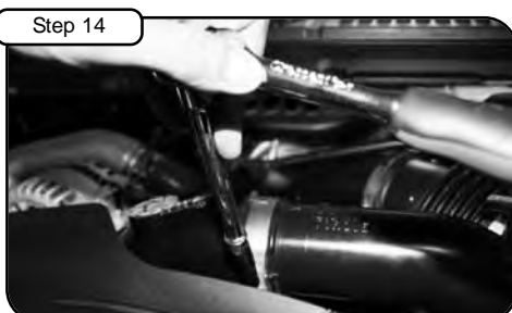
Tighten clamp using 7/16" nut driver. See Notes 2 & 4.
