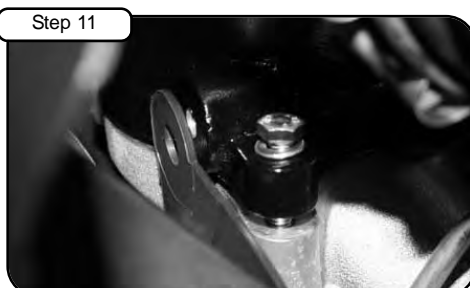
Using M6 x 1.00 x 25 screw and washer secure last remaining manifold mount and tighten. Tighten all screws and nuts using 10mm socket or wrench. See Notes 2 & 5.
