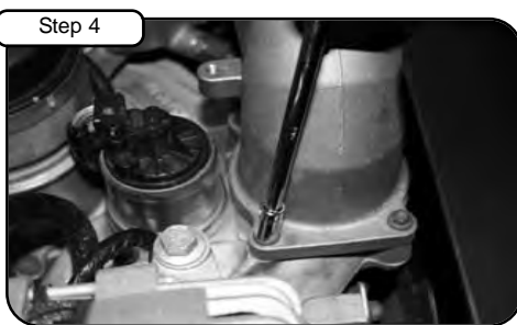
With 8mm socket and extension loosen 4 screws holding in manifold.
