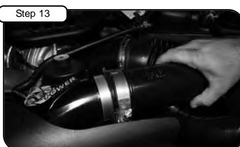
Re-attach intercooler tube to manifold.
