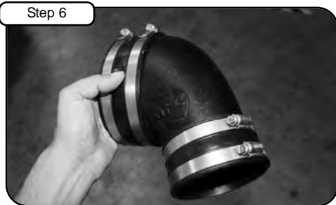
Install couplers with clamps provided to tube. Do not tighten clamps at this time.
