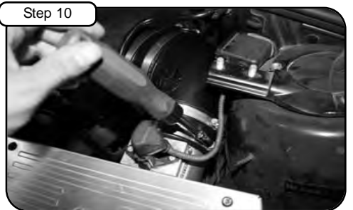
Tighten clamps on adaptor side using 5/16" nut driver.
