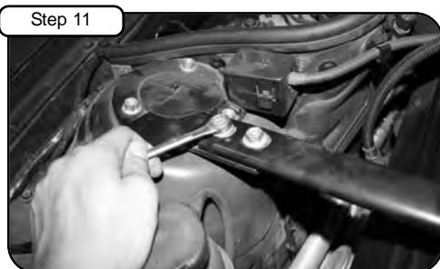
Re-install strut brace and tighten all 4 nuts using 13mm socket or wrench.
