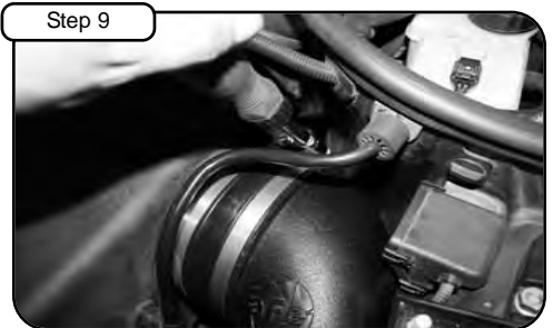
Adjust couplers for proper engagement, then tighten clamps on intake plenum box using 5/16" nut driver.
