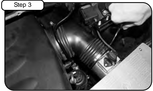
With 1/4" nut driver loosen clamps on stock intake tube.
