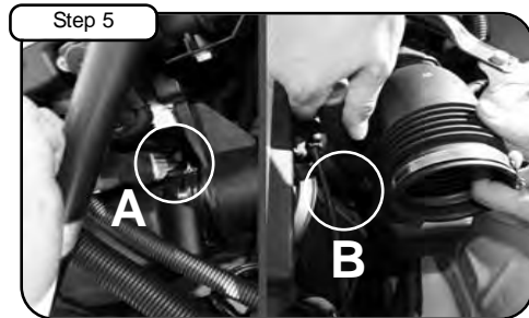
Step 5 A) Loosen clamp on back of tube attached to smog pump. B) Loosen clamp on Throttle Body using 1/4" nut driver.
