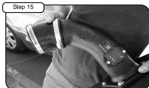
Step 15 Attach coupler to tube with clamps provided. Do not tighten.
