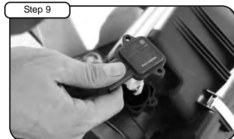
Step 9 Carefully remove MAF sensor.
