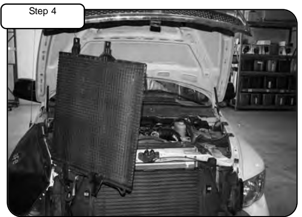
Step 4 With A/C condenser turned 90 degrees, secure to the vehicles lifted hood using steel wire.
