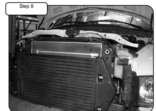
Step 8 Remove the upper radiator support and set aside on top of fan shroud. Loosen clamps on intercooler tubes using 7/16" deep socket. Now remove stock intercooler and factory couplers/clamps out of vehicle. Turn over to page 2 →
