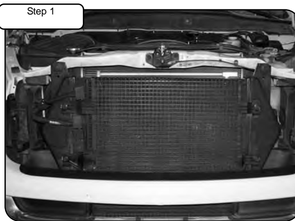
Step 1 Stock Intercooler. NOTE: Disconnect battery before install. Remove stock air box or intake system from vehicle for easier installation.
