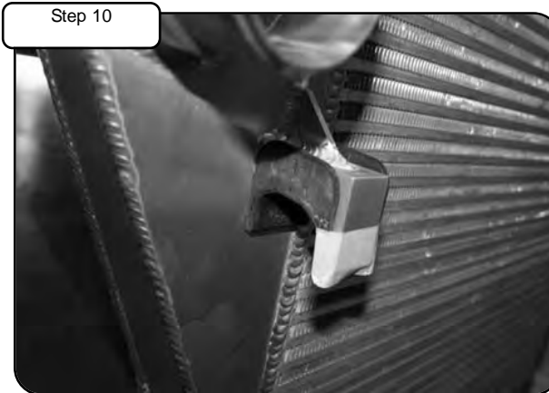
Remove the U-shaped rubber isolators from stock intercooler and install to new BladeRunner® intercooler. NOTE: Tape isolators in place for easier installation.
