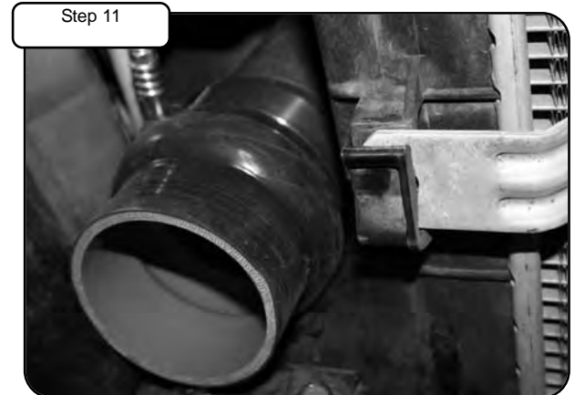
Install new silicone hump couplers and new clamps provided to intercooler tubes. Tighten and torque clamps on intercooler tubes to 5ft. lbs. Now install BladeRunner® intercooler into vehicle.
