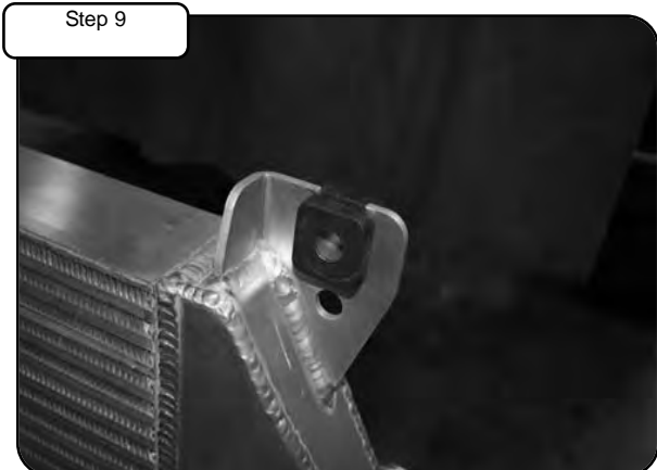
Remove the two upper-rubber isolators with spacers from stock intercooler and install to new BladeRunner® intercooler.
