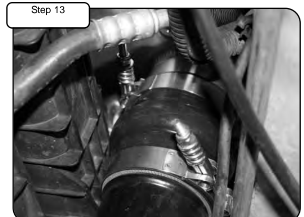
INTERCOOLER MAY NEED ALIGNMENT, TIGHTEN WHEN IN CORRECT POSITION & PROPER CLEARANCE. Re-install Radiator support (See reverse steps 5 through 8). Tighten and torque all clamps to 5 ft. lbs. Re-install A/C condenser to new intercooler using new M8 screws and lock washers provided and tighten.
