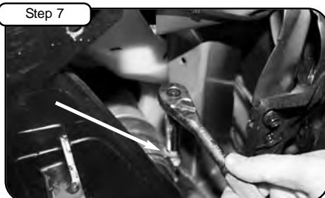
With 7/16" nut driver, loosen clamp on intercooler.
