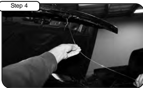
Using bailing wire or bungee cord, secure condenser to grill.
