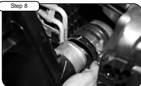
Pull back coupler from intercooler.
