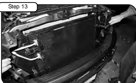
Re-install intercooler to radiator support. (step 5) Re-attach a/c condenser and cover and tighten. (step 2)
