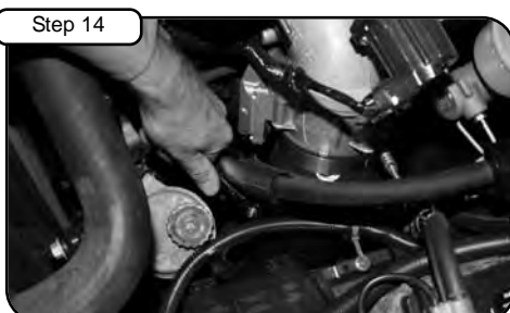
Tighten all four clamps. Make sure all clamps are completely tighten. Check and tighten after 50 miles!
