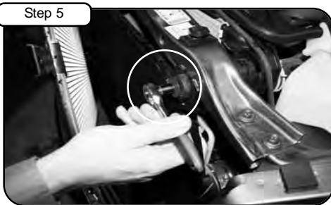
Loosen the two 10mm screws holding in intercooler on radiator support.
