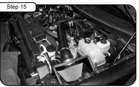
Step 15 Your Intake is now complete. Please check all clamps periodically and tighten as needed. Thank you for choosing aFe power.
