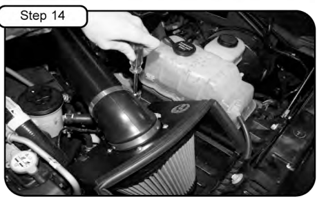
Step 14 Position tube and tighten all clamps using 5/16" nut driver. Re-connect MAF sensor harness.
