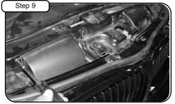
Secure using the 4 screws removed in step 2. Tighten using T25 Torx bit
