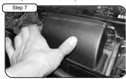
Re install the passenger ram air duct.
