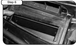
Verify that both D.A.S. Scoop tabs sit flush against mounting surface.
