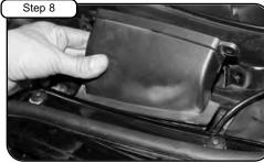
Re install the driver ram air duct.
