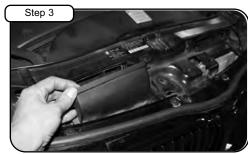
Remove passenger and driver side ram air duct from vehicle
