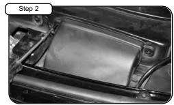
Remove both the passenger and driver side ram air ducts. Ram air ducts are secured with 2 T25 torx screws.(Save for later installation)
