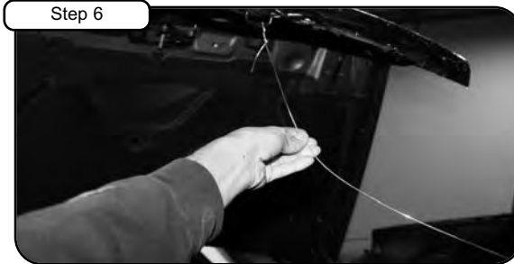
Step 6 With A/C condenser turned 90 degrees, secure to the vehicles lifted hood using steel wire.
