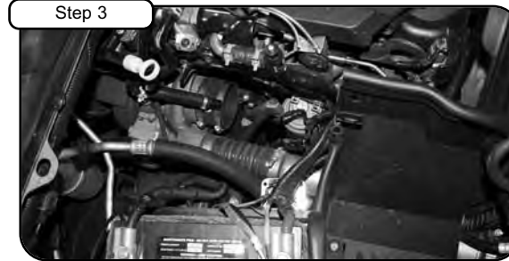
Step 3 Loosen clamp on intercooler inlet tube using 7/16" deep socket. Do not damage the coupler hose that attaches to the turbo, as it will be re-used.
