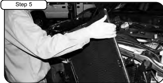
Step 5 Rotate the A/C condenser up and out away from vehicle. Take care to prevent damage to A/C lines.
