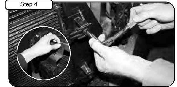
Step 4 Remove plastic A/C line protector on passenger side. With 13mm socket or wrench loosen the 4 bolts holding in A/C condenser.
