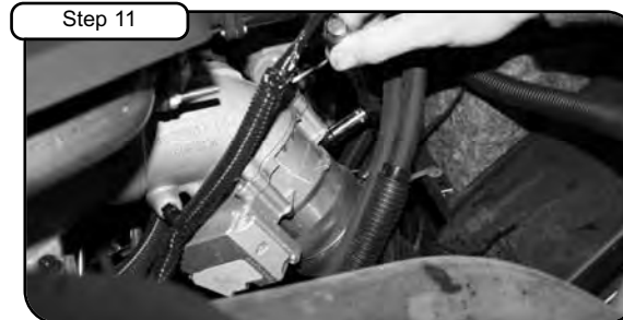
Step 11 With 7/16" deep socket, loosen clamp on manifold. Push down on intercooler tube and disconnect from manifold.
