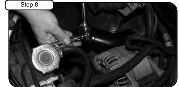
Step 8 With 10mm socket and extension loosen the two bolts holding in radiator on back of upper radiator support.
