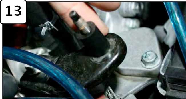
With provided nylon spacer, place on air box mounting point.
