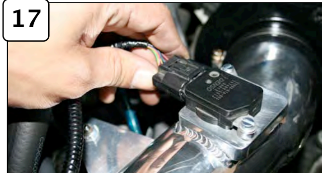
Tighten all clamps using 5/16" nut driver. Re-connect MAF sensor harness and battery terminals.
