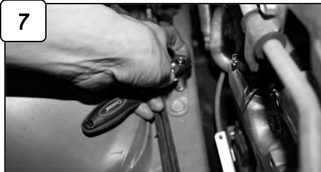
7 With 12mm socket or wrench loosen the bolt on frame and save for install of housing tab.
