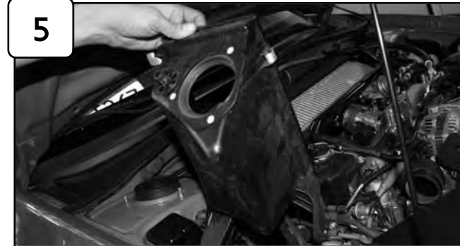
5 With 12mm socket or wrench, loosen the 2 bolts securing bottom half of air box and remove.
