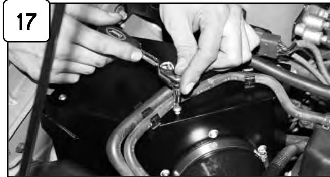
Install cover and tighten using 4mm allen key. Attach vacuum lines to cover tabs.
