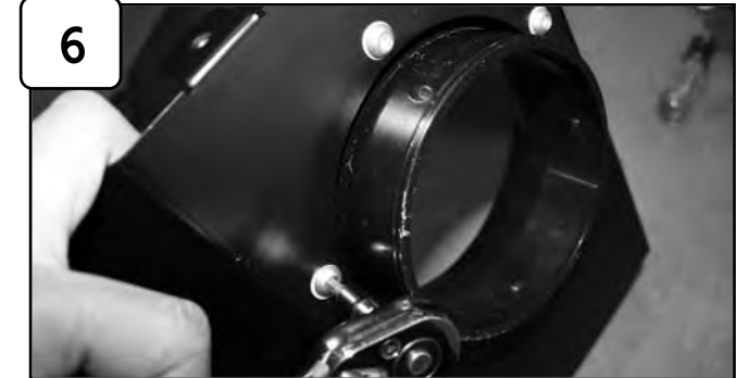
6 Install filter adaptor to housing using supplied button head screws and wavy washers. Tighten using 4mm allen key.
