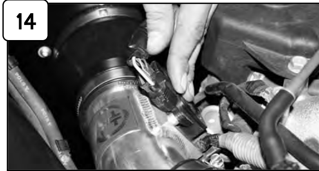
Re-connect MAF sensor harness.
