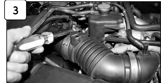
3 Disconnect MAF sensor. Loosen clamps on intake tube using 5/16" nut driver.
