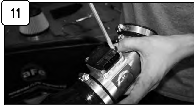
Install MAF sensor on intake tube using M4 screws provided. Attach couplers with clamps to intake tube.
