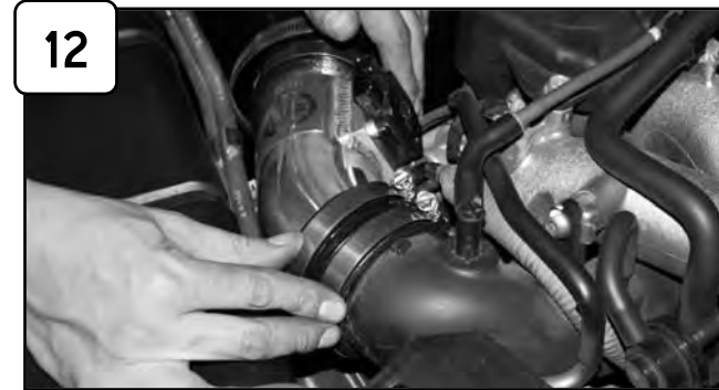
Install and position new tube to throttle body and filter adaptor.
