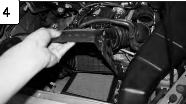
4 Pull back vacuum lines on top of air box. Remove upper half of air box with intake tube.
