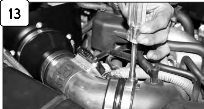
Tighten all clamps using 5/16" nut driver.
