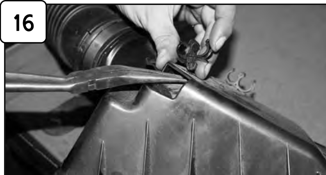
Remove clips from upper half of air box. Attach onto new cover.
