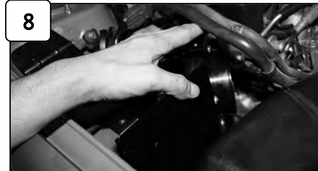
8 Install housing into vehicle and position tab to frame and bolt from step 7. Tighten using 12mm socket or wrench.
