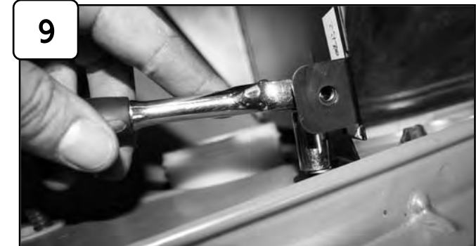
9 With screw and washer provided, tighten top of housing tab to inside of fender using 10mm socket or wrench.
