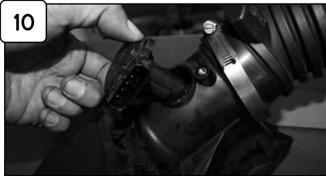
Remove MAF sensor from stock intake.
