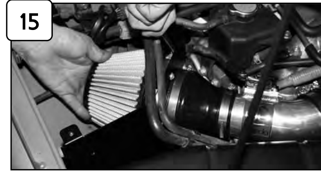
Install air filter and tighten using 5/16" nut driver.
