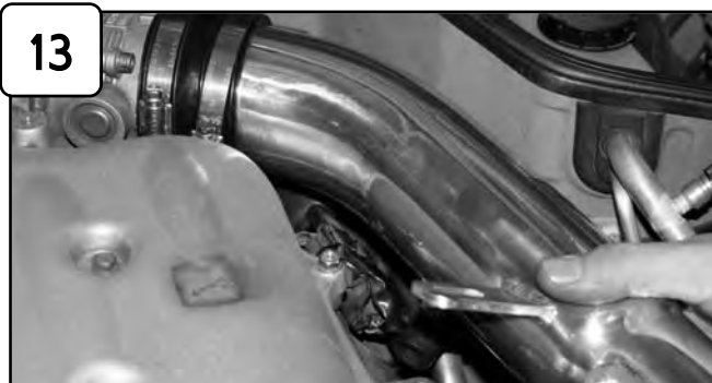
Insert tube into couplings. Locate hole on tab to mounting location on engine plenum.
