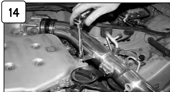
Secure tube and tighten using M6 screw and washer provided. Tighten using 10mm socket or wrench.
