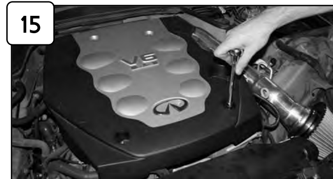
Re-install engine cover and tighten using 10mm socket or wrench.
