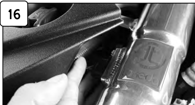
Reconnect MAF sensor harness.
