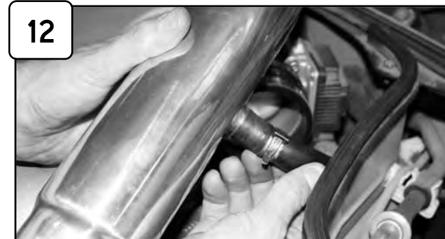
Attach crank case line to intake tube.
