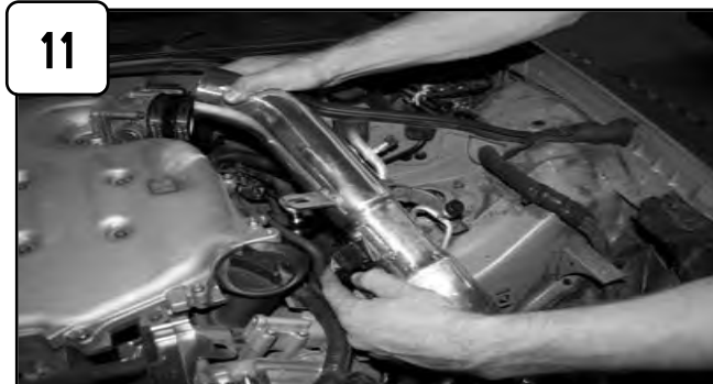
Align intake to coupler on throttle body and bracket location.
