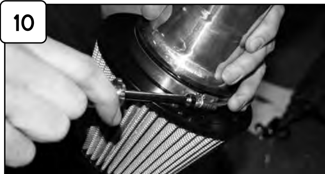
Install air filter to intake tube and tighten using 5/16" nut driver.
