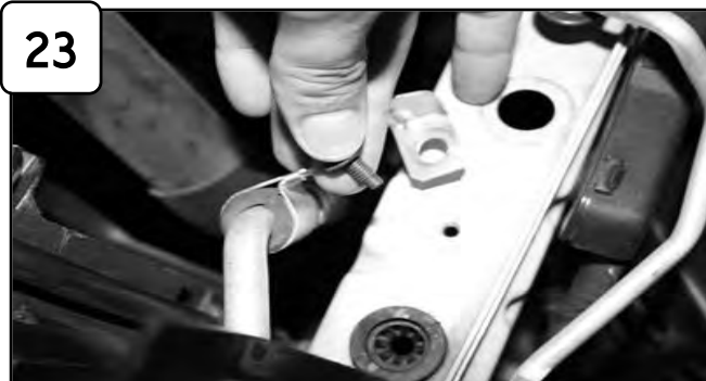
Loosen bolt holding in radiator fan & A/C bracket with 10mm socket or wrench. (To be used in step 24A) Loosen bolt holding in radiator fan bracket with 10mm socket or wrench. (To be used in step 24C.)
