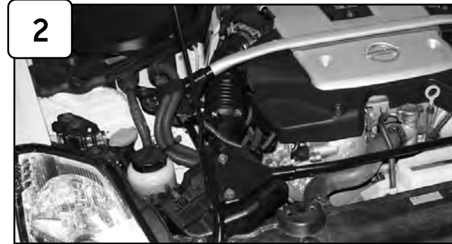
Complete Stock passenger intake. Please disconnect battery terminals before installation.
