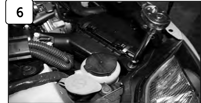
Loosen clamps using 5/16" nut driver. Loosen bolt holding in tube with 10mm socket or wrench. Pull back crank case line from vent box.
