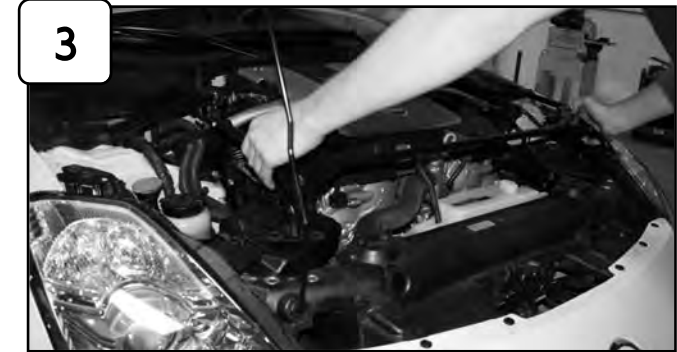
NISMO 350Z only , remove front strut brace before installation.
