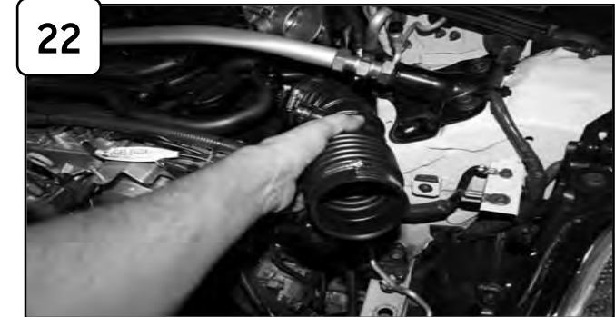
Remove complete intake out of vehicle.
