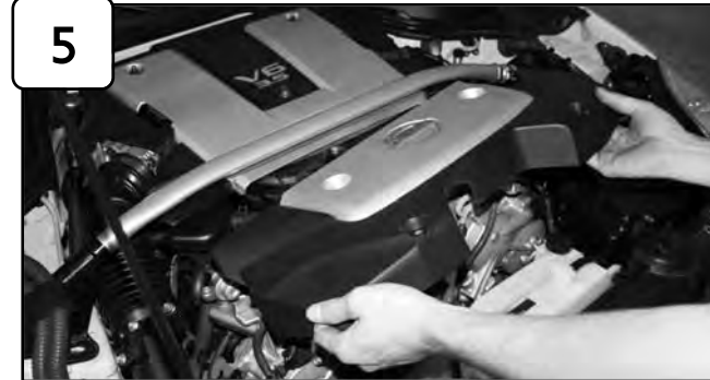
With 10mm socket or wrench, loosen the 5 bolts holding in engine cover and remove.
