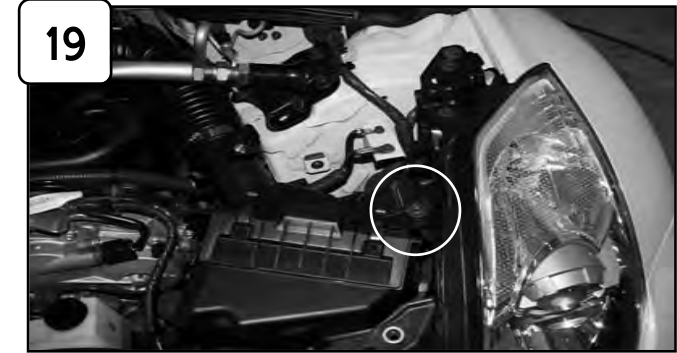
With 10mm socket or wrench, loosen the bolt holding in air box.
