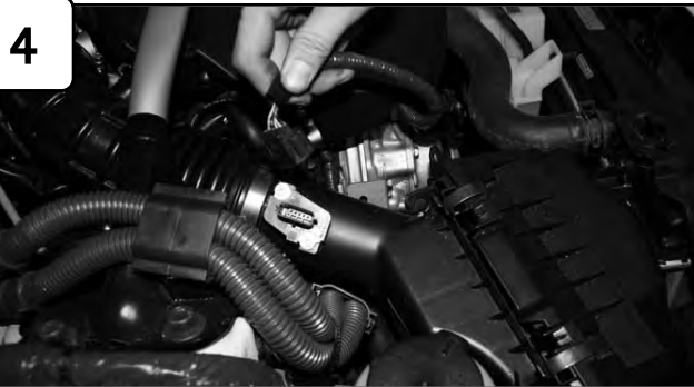
Disconnect MAF sensor harness.
