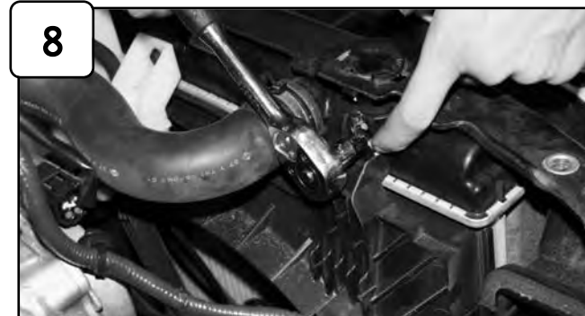
Loosen bolt holding in radiator fan bracket with 10mm socket or wrench. (To be used in step 9C.)
