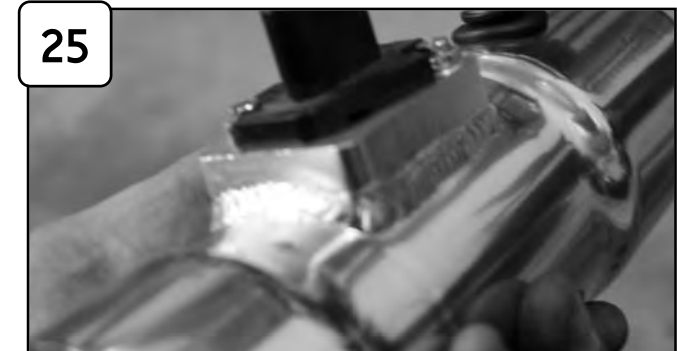
Remove MAF sensor from stock air box. Install into new tube with M4 screws provided and tighten using flat head screwdriver. Install rubber grommet to tube provided.
