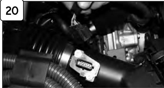
Disconnect MAF sensor harness.
