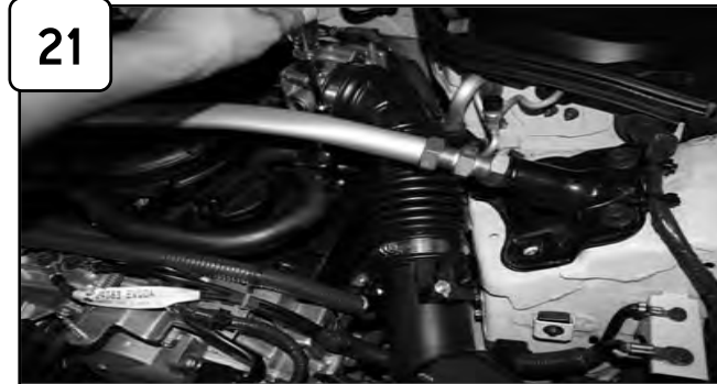
Loosen clamps using 5/16" nut driver. Pull back stock intake tube from vent box.
