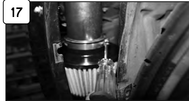
17 Install air filter and tighten using 5/16" nut driver. Attach pre filter to filter if desired. Re-install plastic fender well and re-connect battery terminals.
