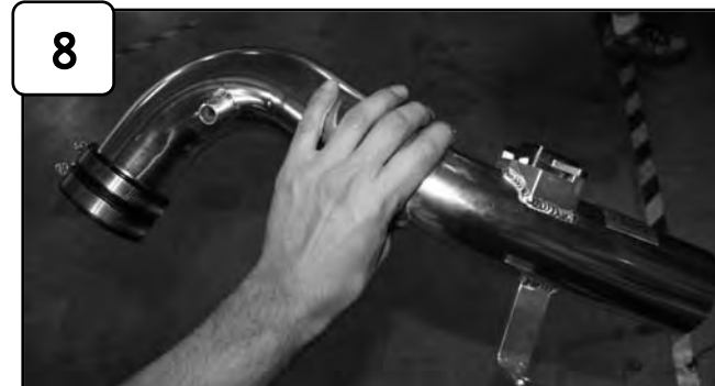
8 Install upper intake tube assembly into vehicle with provided 05-00417 coupling and clamps. Do not tighten.
