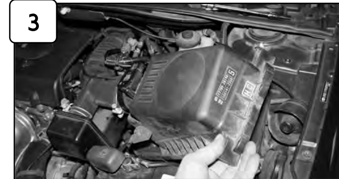
3 Disconnect MAF sensor and loosen clamp using 10mm socket or wrench. Unclip upper half of air box and remove. With phillips screwdriver loosen VSV module from tube. Loosen clamp with pliers on throttle body and remove stock intake tube.
