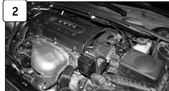
2 Complete Stock intake. Please disconnect battery terminals before installation.
