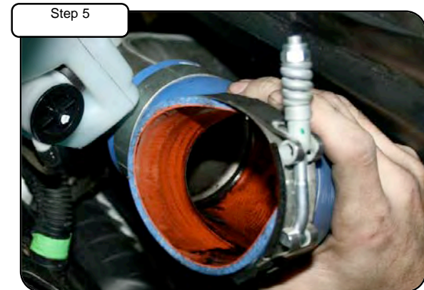
Remove the stock intercooler tube through the fender well.
