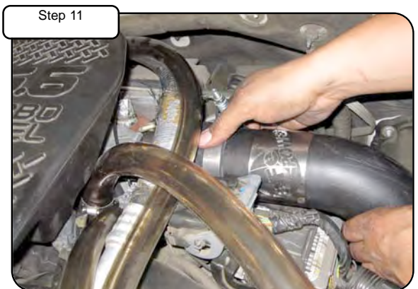
Install the silicone reducer coupler provided onto turbo housing. Install intercooler tube into coupler. Do not tighten clamps so the tube can move and flex to ease installation of coupler at intercooler inlet.
